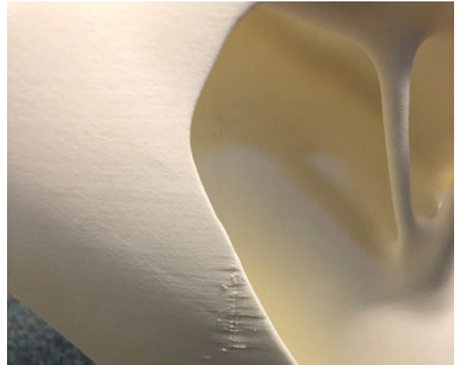
FIGURE 1 Recoater Failure Initiated Part Failure
