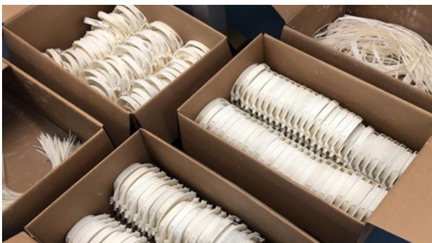
FIGURE 2 Overview of the faceshields serial production before washing, sanitizing and separate packaging
