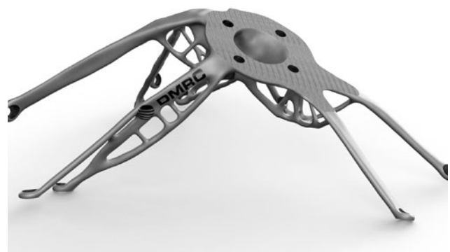
FIGURE 2 AM Designed Reaction Wheel Bracke
