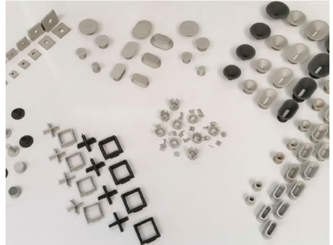
FIGURE 2 Process-related design limitations that illustrate the need of a support material
