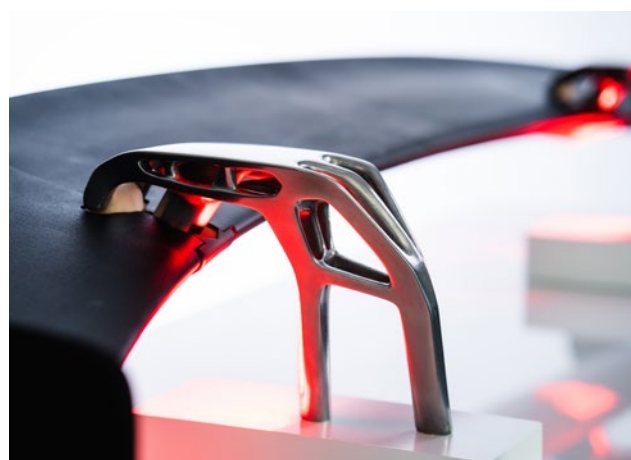
FIGURE 1 Rear wing bracket "Wing3D" [Source: EDAG Engineering]
