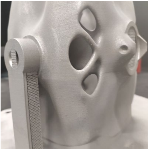
FIGURE 1 Gimbal built with high speed parameter
