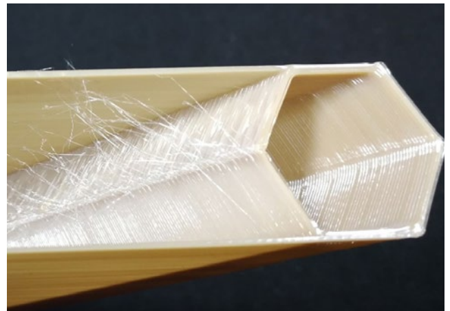
FIGURE 2 Typical FDM error pattern oozing / stringing
