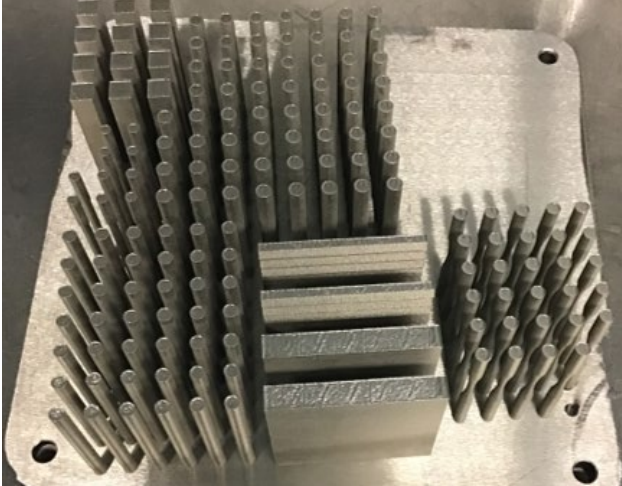
FIGURE 1: Standard build job for microstructural and mechanical characterization for the three addressed materials Ultimet, 36NiCrMo16 and W360.
