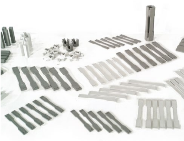
FIGURE 1 Specimens manufactured in the Metal-FDM process
