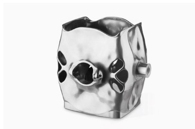
FIGURE 2 Component after final surface finish through vibratory grinding
