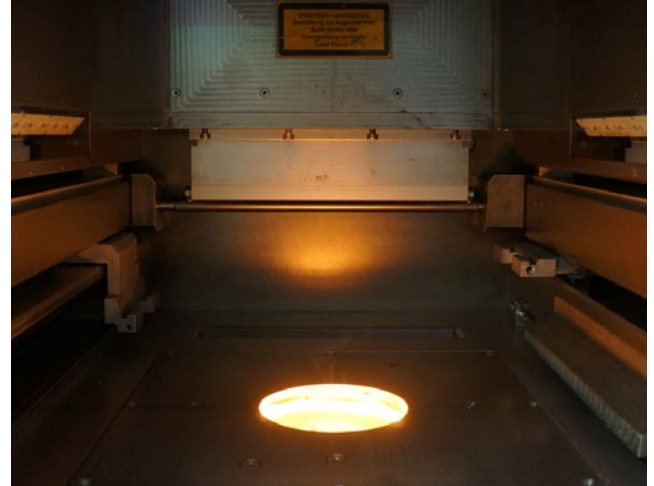
FIGURE 2: Installation of the IR build room heater in the SLM Solutions 280 HL.
