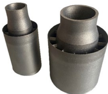
FIGURE 3 Successfully built, crack-free Rotor consisting of Stellite 6
