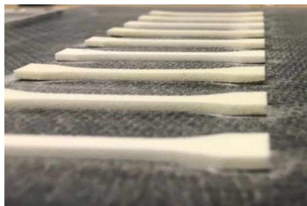
FIGURE 2 Tensile bars directly built on building platform
