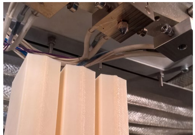
FIGURE 3 Custom built specimen in a build chamber of an FDM machine
