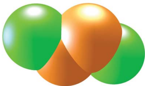
Figure 11. Present molecular interaction model for 1,2-dichloroethane. The green spheres represent chlorine atoms, the brown spheres represent methylene groups. Note that the sphere diameters correspond to the Lennard-Jones size parameters, which are depicted according to the molecular geometry scale.
