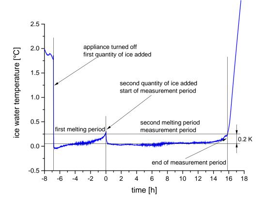
Fig. 5 Ice water temperature over time.
