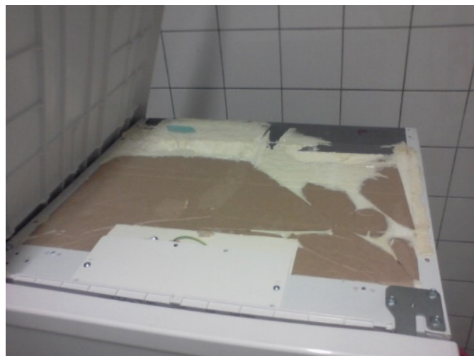
Figure 8: Missing diffusion barrier at the cabinet of appliance F01.
