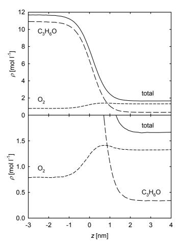
**Fig. 4** Total density and partial density profiles of the mixture oxygen + acetone at 400 K and  $x_{O2} = 0.05 \,\text{mol mol}^{-1}$  across the VLE interface at two different scalings. — total density; —— partial density of oxygen; —— partial density of acetone.
