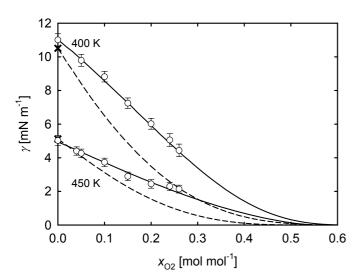
**Fig. 12** Surface tension over the oxygen mole fraction of the liquid bulk phase  $x_{\rm O2}$  at 400 and 450 K for the mixture oxygen + acetone.  $\bigcirc$  molecular dynamics, this work;  $\times$  correlation of experimental data, Mulero et al.; <sup>46</sup> --- parachor method; — fit of eq. (6) to the present molecular simulation data. The statistical uncertainties of the simulation data are given as the standard error on a 95 % confidence interval.
