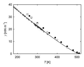
**Fig. 9** Surface tension over temperature for acetone.  $\bigcirc$  molecular dynamics, this work;  $\bullet$  density functional theory, Klink and Gross;  $^{44}$  — correlation of experimental data, Mulero et al.;  $^{46}$  + experimental data.  $^{37-42}$  The statistical uncertainties of the simulation data were considered as the standard error on a 95% confidence interval and are only visible if they exceed the symbol size.
