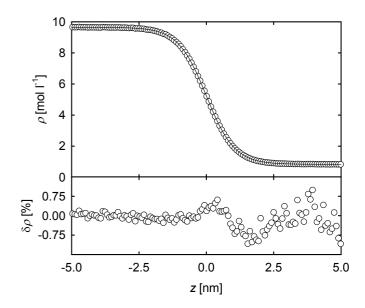
**Fig. 1** Density profile and deviations from the fitting function in case of acetone at 450 K through the VLE interface.  $\bigcirc$  simulation results; — fit of eq. (1) to the simulation results. The deviations are given as  $\delta \rho = (\rho - \rho_{\rm fit})/\rho_{\rm fit}$ .
