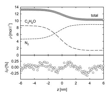
**Fig. 8** Total and partial density profiles as well as deviations from the fitting function through the VLE interface of the mixture nitrogen + acetone at 400 K and  $x_{\rm N2}=0.32\,{\rm mol\,mol^{-1}}$ .  $\odot$  total density and deviations from the fitting function; —— partial density of nitrogen; —— partial density of acetone; —— fit of eq. (1) to the simulation results. The deviations are given as  $\delta\rho=(\rho-\rho_{\rm fit})/\rho_{\rm fit}$ .
