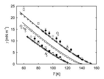
**Fig. 10** Surface tension over temperature for oxygen and nitrogen and their mixture with equimolar liquid bulk phase. ○ molecular dynamics, this work; ● molecular dynamics, Neyt et al.;<sup>51</sup> --- parachor method; — correlation of experimental data, Mulero et al.;<sup>46</sup> + experimental data. <sup>53-55</sup> The statistical uncertainties of the simulation data were considered as the standard error on a 95 % confidence interval and are only visible if they exceed the symbol size.
