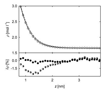
**Fig. 5** Total density profile and deviations from the fitting functions for the mixture oxygen + acetone at 400 K and  $x_{\rm O2} = 0.05\,{\rm mol\,mol^{-1}}$  on the vapor side of the VLE interface.  $\odot$  simulation results; ——,  $\odot$  fit of eq. (1) to the simulation results and their deviation; —,  $\odot$  fit of eq. (2) to the simulation results and their deviation. The deviations are given as  $\delta\rho = (\rho - \rho_{\rm fit})/\rho_{\rm fit}$ .
