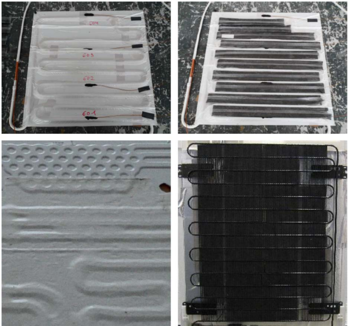
Fig. 1 Foamed evaporator of K-12020S-1 (top, left), equipped with PCM elements (top, right), rollbond evaporator of K-32122i equipped with PCM foil (bottom, left), condenser of K-32122i equipped with PCM elements (bottom, right)
